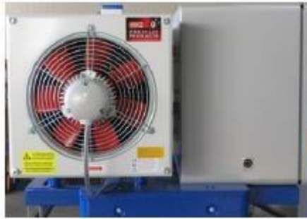
Fig.2: Fan at air inlet.
